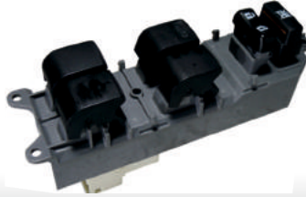
AN 1402 TOYOTA HILUX / CAMRY YENİ MODEL 1999-> TOYOTA COROLLA 2006-> DÖRT CAM ANAHTARI OEM NO : 8482006100 / 8482042190
