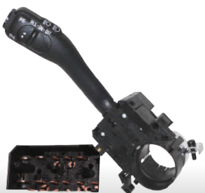
VW 16 VW.GOLF IV 1997->2004 / VW.BORA 2000->2005 VW. PASSAT B5 / B6 1997->2005 SEAT TOLEDO II / LEON II 1999-> 2005 SKODA FABIA / OCTAVIA 2002->2010 AUDI A3 1997->2003 / AUDI A6 1997->2001 SİNYAL KOLU CRUISE KONTROLLU OEM NO : 8L0953513H / 8L0953513H01C / 8L0953513J / 8L0953513J01C
