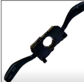
VW 16 VW.GOLF IV 1997->2004 / VW.BORA 2000->2005 VW. PASSAT B5 / B6 1997->2005 SEAT TOLEDO II / LEON II 1999-> 2005 SKODA FABIA / OCTAVIA 2002->2010 AUDI A3 1997->2003 / AUDI A6 1997->2001 SİNYAL KOLU CRUISE KONTROLLU OEM NO : 8L0953513H / 8L0953513H01C / 8L0953513J / 8L0953513J01C
