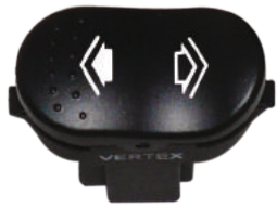
AN 0910 FORD TRANSIT V347 / FORD FOCUS YENİ MODEL TEKLI OTOMATİK CAM ANAHTARI OEM NO : 1060717 / 1066699 / 1073473 / 1324939 / 98AB14529DA / 98AB14529DB / 98AB14529DC / 98AB14529DD
